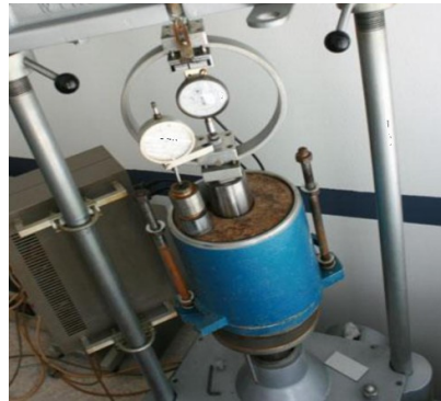
Fig -4: CBR loading on a reinforced soil sample
