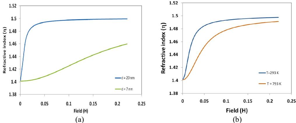
Fig.1. (a) the variation in refractive index ( $\eta$ ) of particles of two different diameters (7 nm and 20 nm) as a function of magnetic field at constant temperature of 300 K and (b) variation in refractive index ( $\eta$ ) of particle (diameter = 15 nm) at different temperatures, i.e. 293 K and 793 K with magnetic field.
