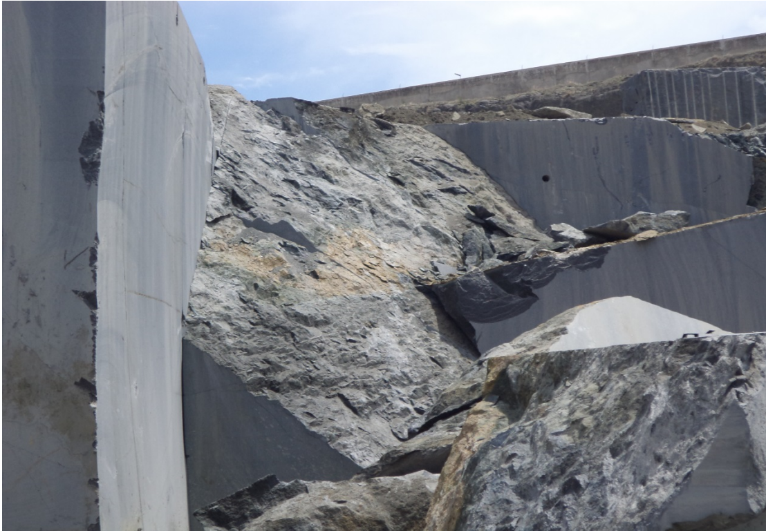
DEFECTIVE SHEAR PLANES WITH NIL PRODUCTION
