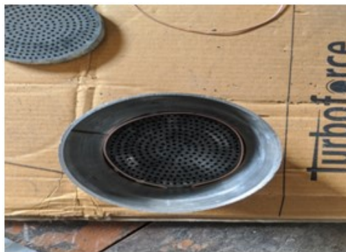
Fig:9 Ceramic disc installation in shell
