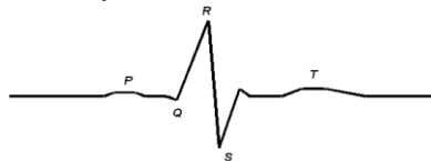
Fig1: Typical ECG waveform with the P, Q, R, S and T waves for one heart beat
