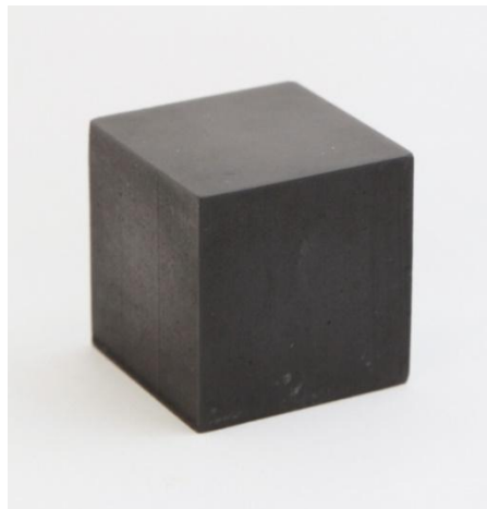
Fig.6:A sample used for the deformation test
